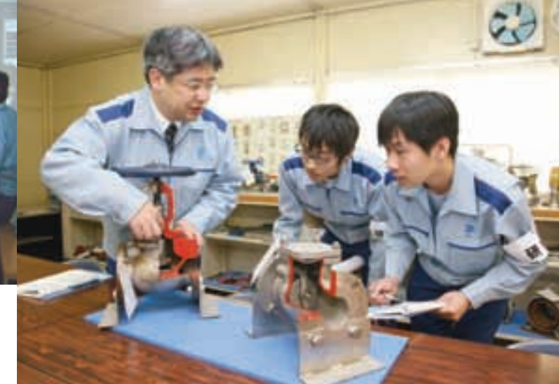
The training room contains cutaway models of various pieces of equipment found in the plant. This enables the trainees to learn the mechanisms of the plant equipment and the maintenance methods.
